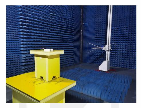
Spurious Emission Test Setup (Above 1GHz)
