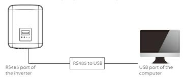
The product is equipped with a Modbus interface via RS485 port. The Modbus interface can be connected via RS485 to USB cable or external Modbus control device to SCADA systems for industrial use and has the following tasks:
