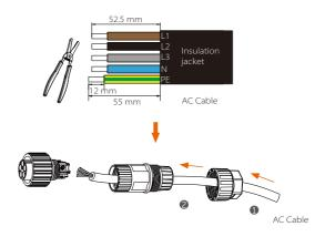
c) Insert the stripped end of the five wires into the appropriate holes of the male insert (The N wire and PE wire must be connected correctly), and then tighten each screw to ensure each wire in place (Use the accompanying inner hexagon spanner).
