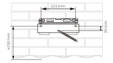
c) Drill holes with  $\emptyset$ 10 drill, make sure the holes are deep enough (at least 60 mm) for installation.
