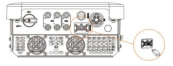
3) Then insert the U-disk into the DONGLE port on the bottom of the inverter. Then turn on DC switch and connect the PV connector, the LCD will show a picture as below.
