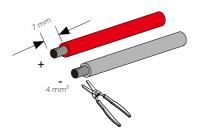
c) Insert the stripped section into positive pin contacts and negative pin contacts, make sure all wires are captured in the pin contacts.
